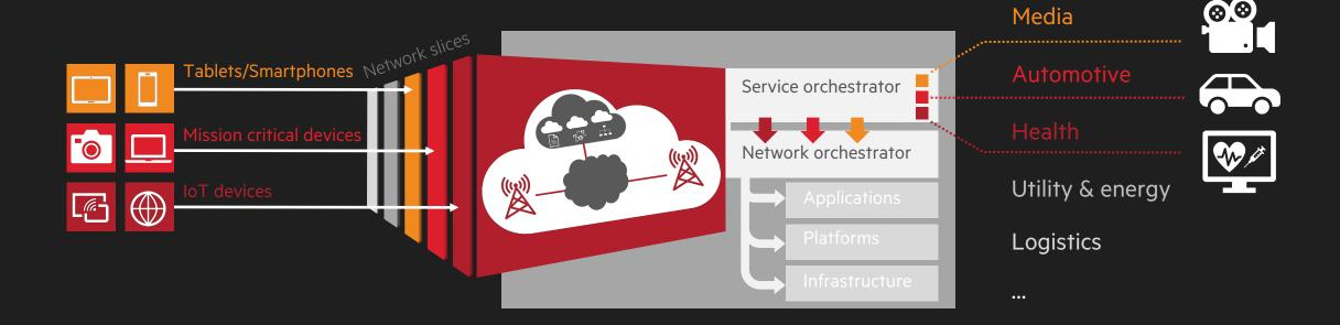
Assignment of devices to network slices
